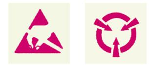
These industry standard ESD symbols are printed on the packing material to notify distributors and users that ESD precautions and proper handling procedures must be utilized to insure the reliability and quality of both the IC's inside as well as the electronic end products that will utilize them.
