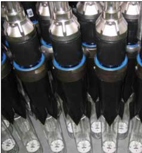
The TrojanUV4000Plus™ has been optimized for disinfection of low quality wastewater using high intensity lamps, and vortex mixers (left) to increase flow turbulence around the lamps. Trojan's UV technology allowed the City of Honolulu, Hawaii to disinfect primary effluent at their Sand Island treatment facility (right), and thereby save hundreds of millions of dollars that would have been required to build secondary treatment facilities.
